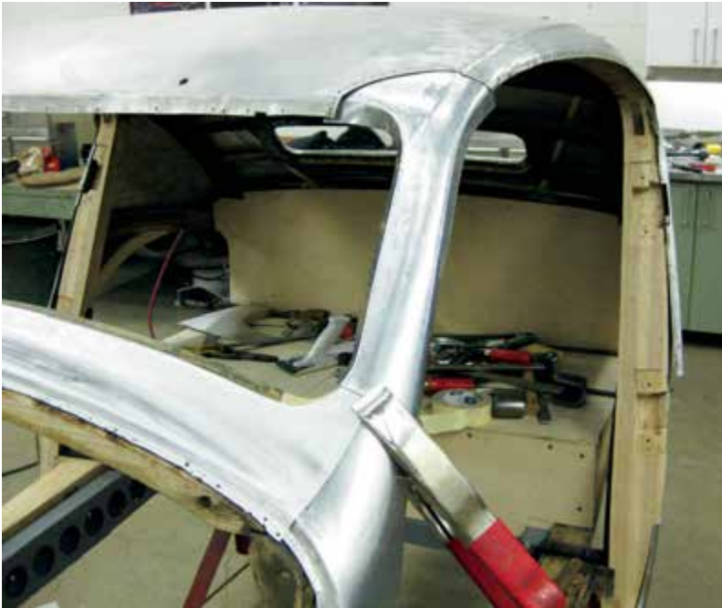
Above: Damaged pieces of the aluminum outer shell are replaced and carefully welded onto the original aluminum.
