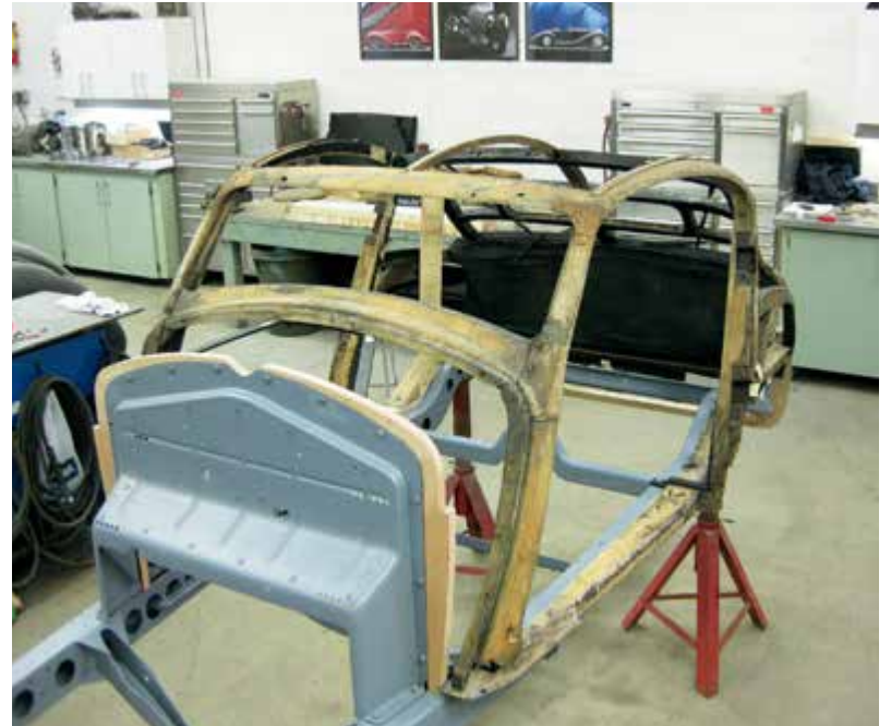
Above: The badly aged wood is replaced while most of the original wooden structure is stabilized and saved.
