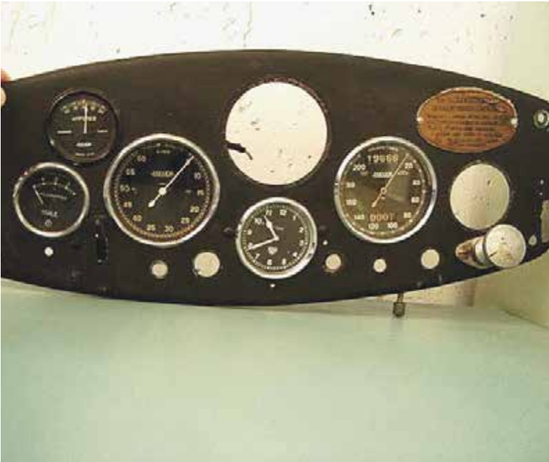
Above: Removal of the brass plaque from the black dashboard revealed the original cracked finish the dashboard would have had before the Greyvenstein restoration.
