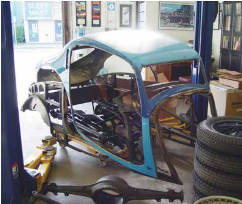
Right: While examining the outer shell of the vehicle, the original two-tone black and cream colours became apparent. These were colour matched and later used on the restored body.
