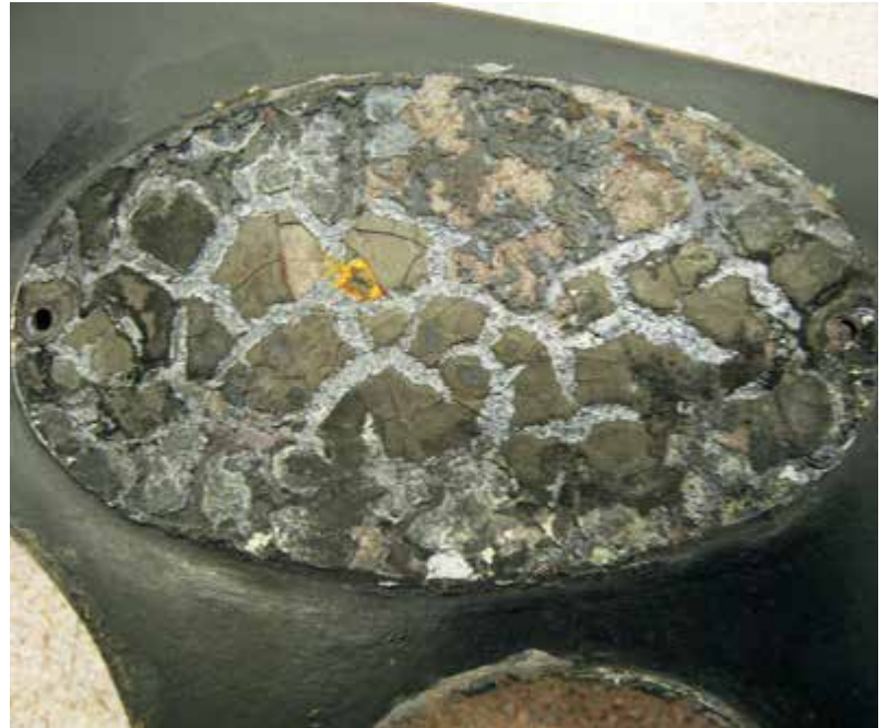
Above: Removal of the brass plaque from the black dashboard revealed the original cracked finish the dashboard would have had before the Greyvenstein restoration.
