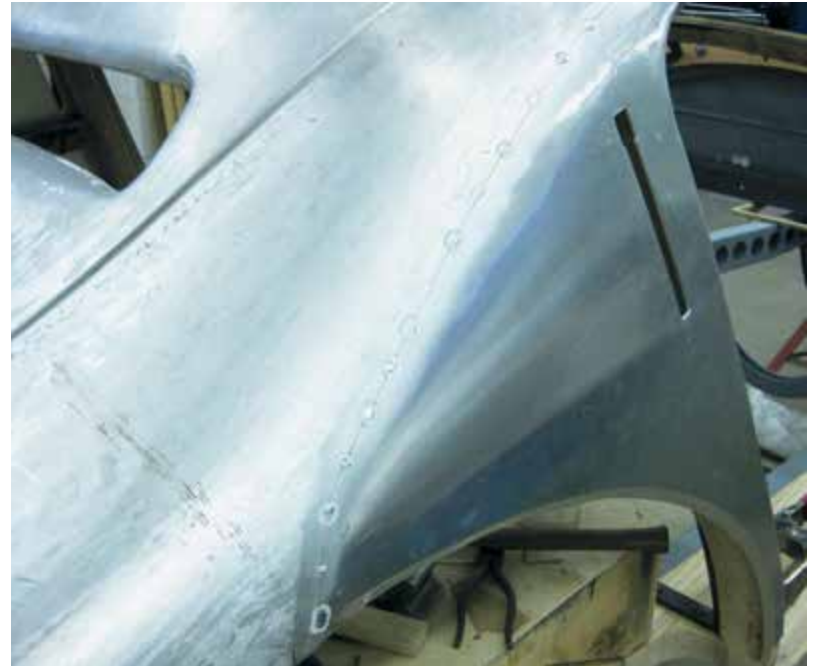
Above: Damaged pieces of the aluminum outer shell are replaced and carefully welded onto the original aluminum.
